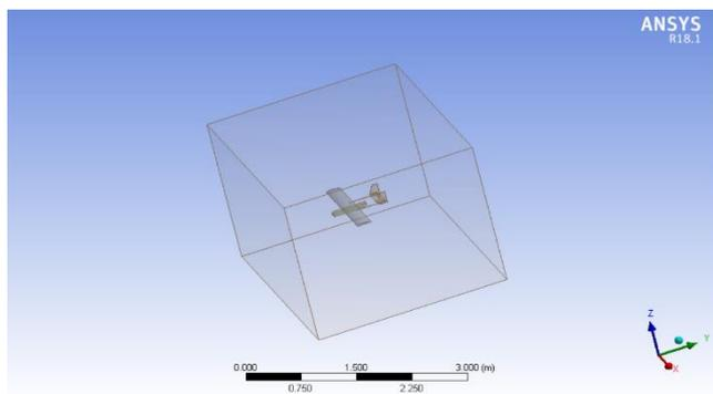
Fig- 13: Model with domain enclosure
