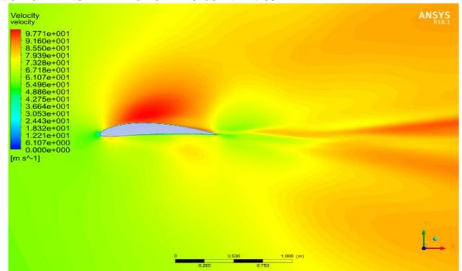
Fig -5: Velocity contour at 35m/s
