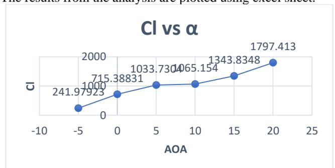
Fig-7: Cl vs  $\alpha$  at 35m/s
