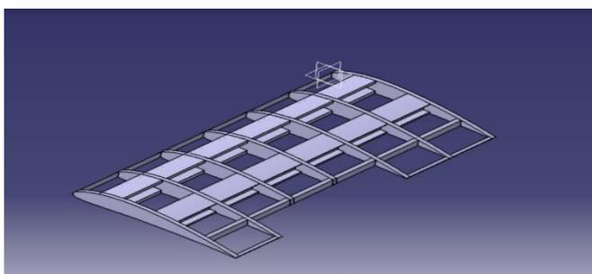
Fig- 18: Wing structures with ribs and spar apart
