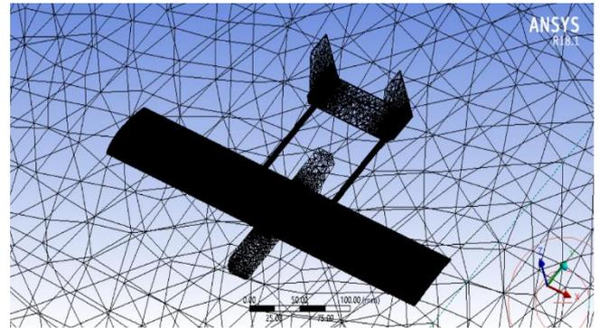
Fig- 14: Complete fine and unstructured mesh
