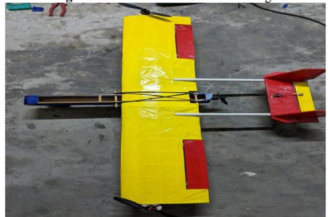
Fig- 27: Final completed VTOL model
