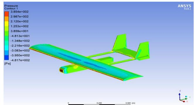
Fig- 15: Pressure contours over the VTOLA
