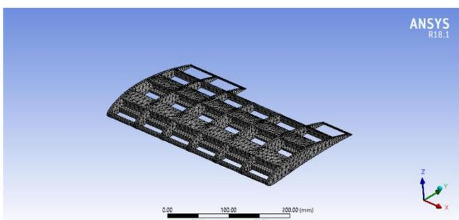
Fig- 19: Mesh of the wing structures with ribs and spar
