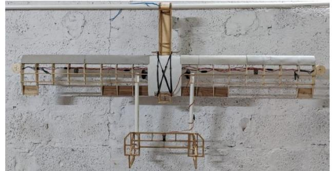
Fig- 26: Structure of VTOL with wirings
