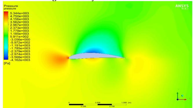
Fig -6: Pressure contour at 35m/s
